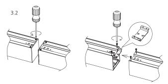
If need to be spliced into series, remove the end cap of each connection side, connect them by connectors and fix by screws.
