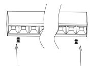
Put the module back and push it into the base, turn on the lamp.
