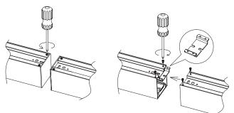
If need to be spliced into series, remove the end cap of each connection side, connect them by connectors and fix by screws.
